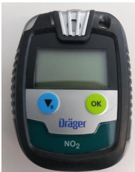
To switch **on** press the OK button and keep your finger on the button for 3 seconds. (You will see the seconds counting down on the reader).
